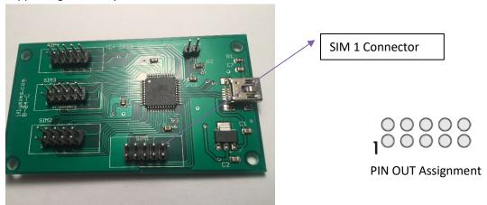
Each Sim Connector is labeled on the Board. There are 4 Sim Connectors labeled SIM 1, SIM 2, SIM 3 and SIM 4.
